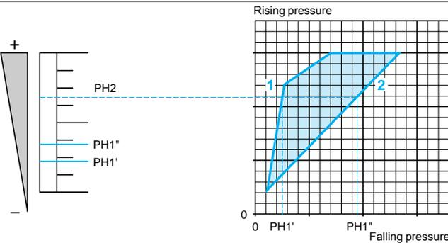
The upper pressure setting at which the pressure or vacuum switch will actuate contact 1 on rising pressure.
