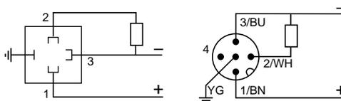
(2) Switch connector pin view
