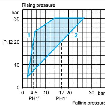
■ Consider a 2nd stage switching point on rising pressure (PH2) of 20 bar (set value at which contact 2 will change state on rising pressure).
