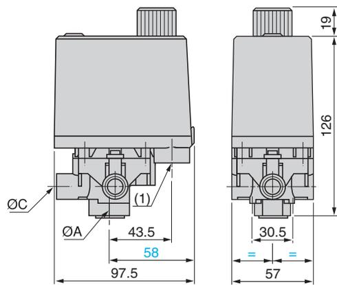
With straight, olive connection, decompression valve
