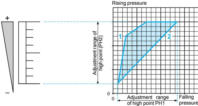
Defined by the difference between the minimum and maximum high point setting values of each stage (PH1 and PH2).
