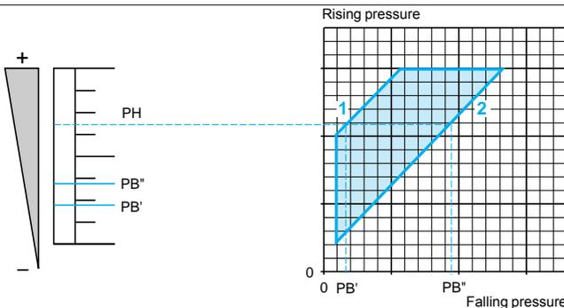
The pressure at which the switch contact changes state on falling pressure.
