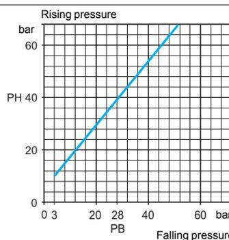
■ Consider a switching point on rising pressure (PH) of 40 bar (set value at which the contact will change state on rising pressure).
