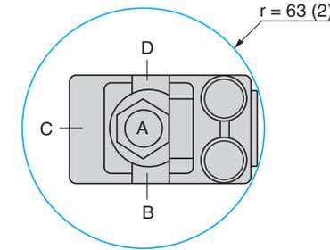
With straight, olive connection, decompression valve
