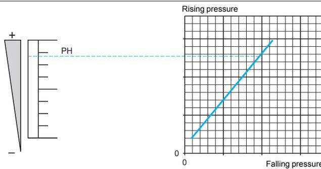
The upper pressure setting at which the pressure or vacuum switch will actuate the contacts on rising pressure.
