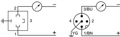
(1) Sensor connector pin view
