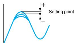
The tolerance between the point at which the switch actuates its contacts and the value indicated on the setting scale. Where very high setting accuracy is required (initial installation of the product), it is recommended to use separate measuring equipment (pressure gauge, etc.).
